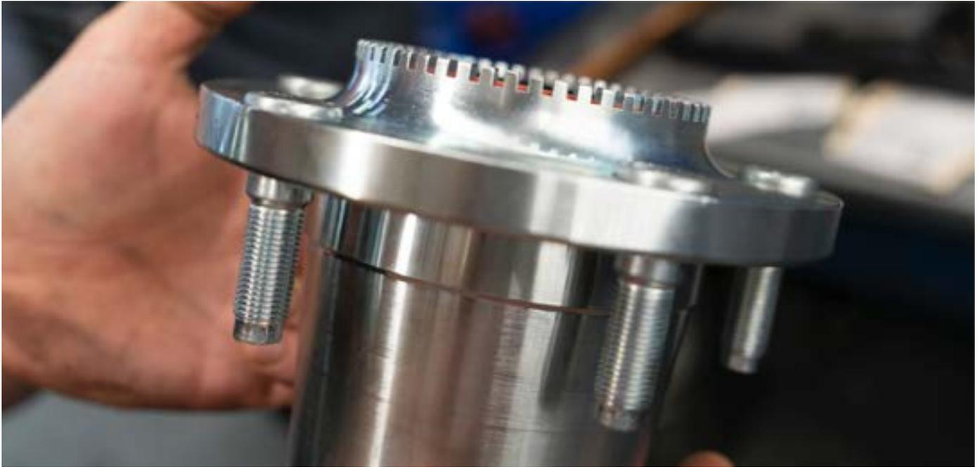
Figure 20. (Seal 0.120-0.160" from top of ABS teeth)
